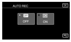
6 Recording starts automatically when the subject within the red frame moves.
