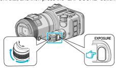
3 Change the numerical value of "APERTURE" by using the adjustment dial.
